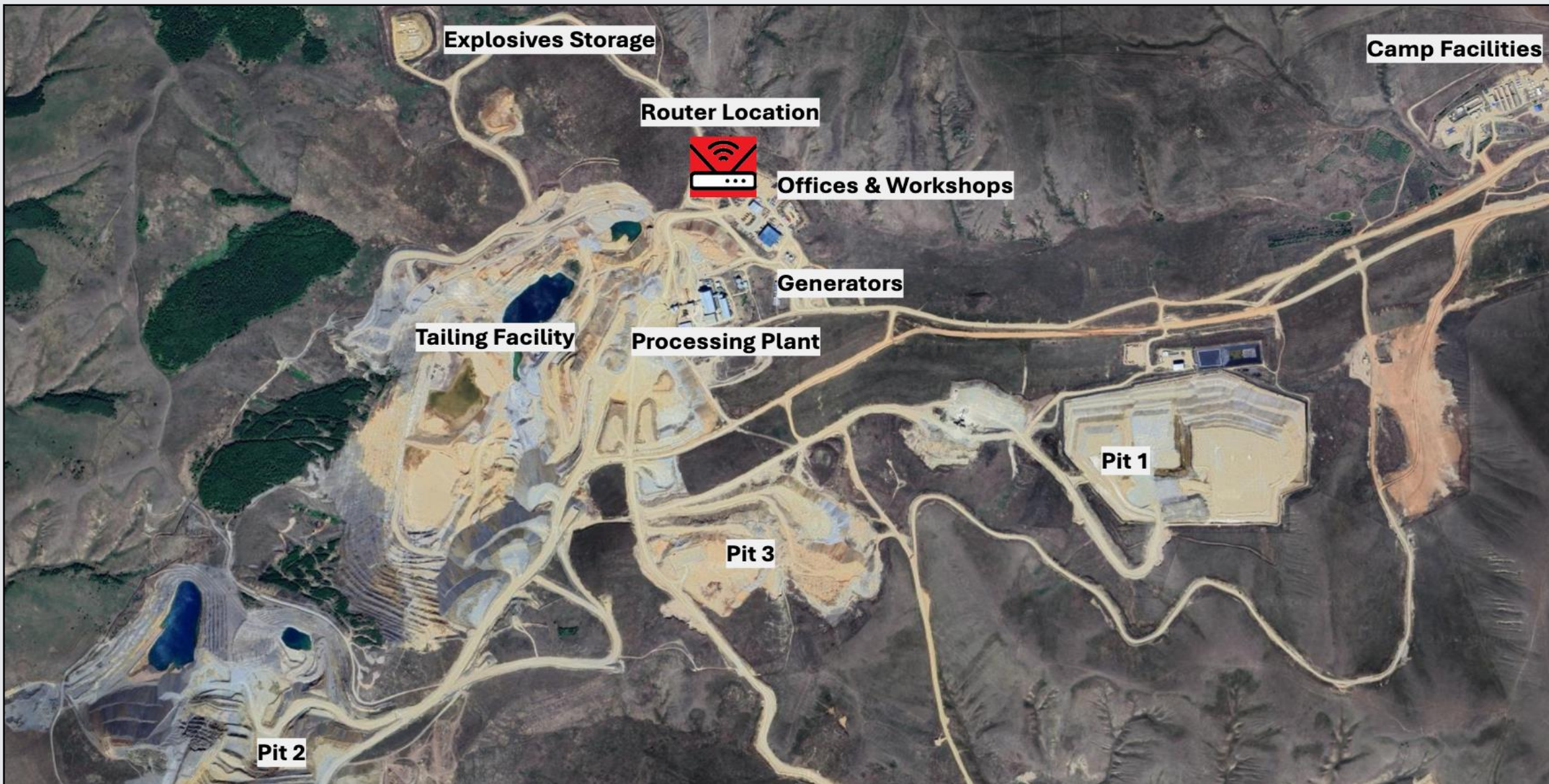
1 ROUTER DEVICE HAS A RANGE OF 10-20 KILOMETERS & CAN COMMUNICATE WITH ALL IOT SENSORS WITHIN THIS RADIUS, EVEN DEVICES LOCATED UNDERGROUND & INSIDE OF STRUCTURES
